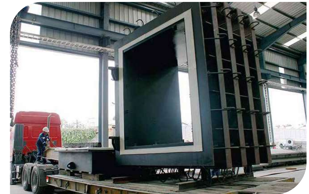
● HIDROELECTRIC PLANT PUCARÁ Watertight Gates
